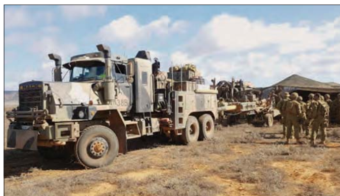
1 CSSB HRV connected to a M777A2 during a Battle Damage Assessment & Repair (BDAR) activity on Exercise Predators Run 2018.
