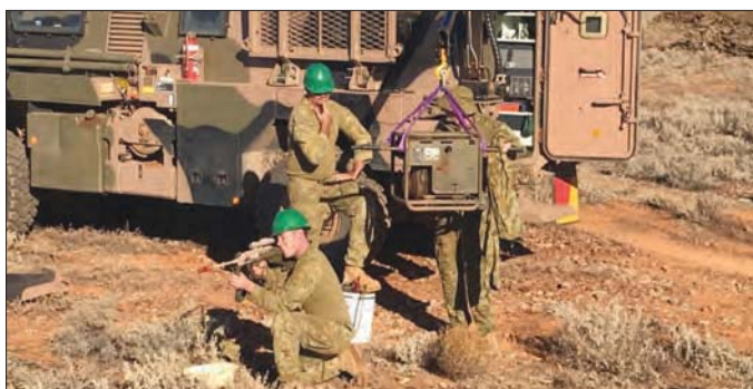
First Exercise with PMGMV using crane to fix 1.3 KVA. CFN Harding providing local defence!
