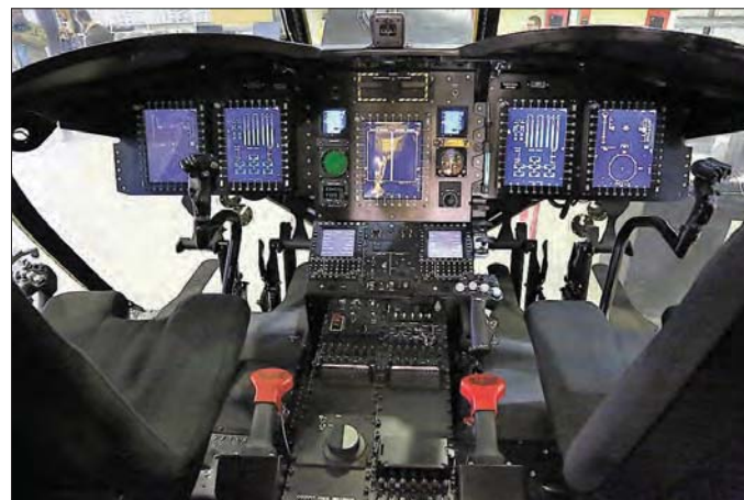
Figure 5: The CAT is a full-scaled avionics simulator.
