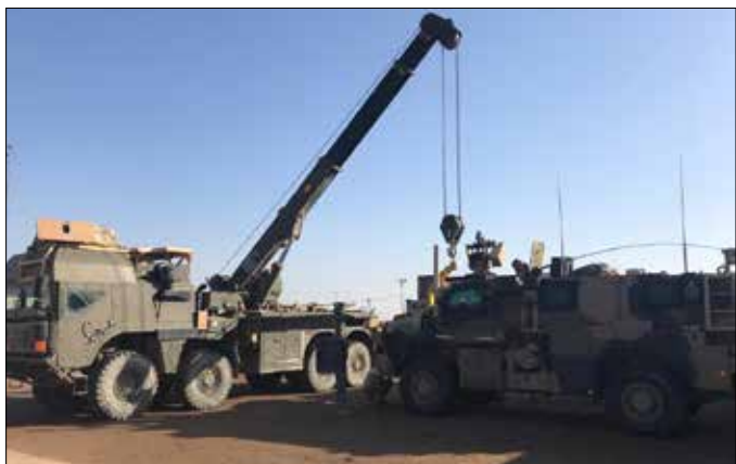
PMV Pack lift with the assistance of the REME HRV
