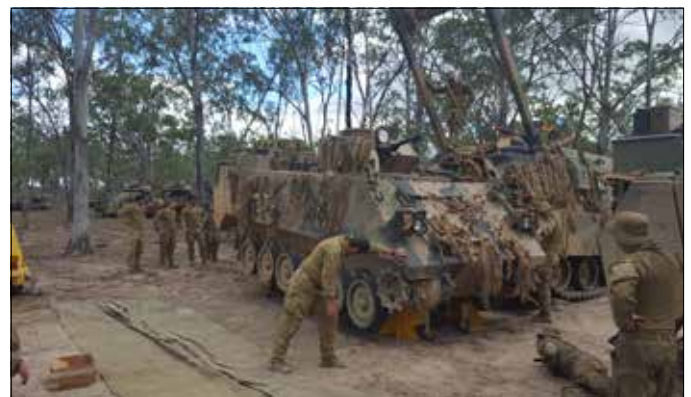
M88 lifting AS4 for servicing
