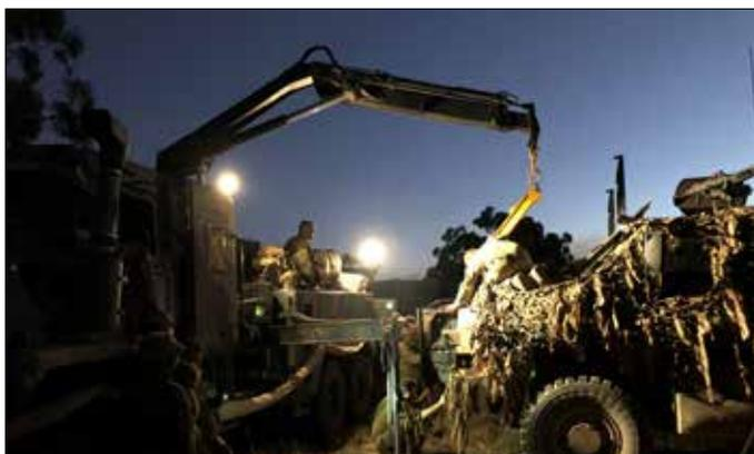
*The A2 conducts a pack lift on a PMV-C to repair an oil leak during EXADLUM.*
