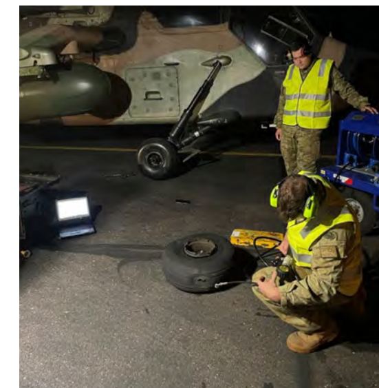
161 TST maintainers replacing a tyre on an ARH Tiger after a heavy landing.
