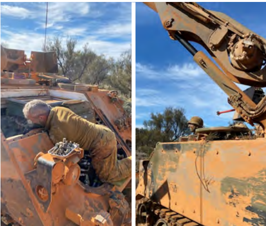
Lima 13 Vehicle technicians replacing a M113AS4 power pack.
