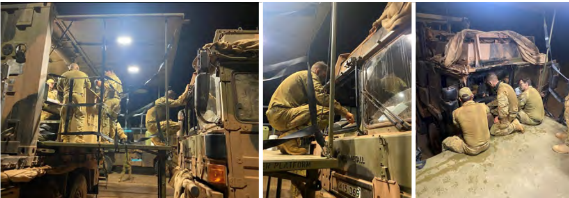
Lima 13 Vehicle technicians replacing a HX77 windscreen, utilising a Maintenance Shelter as the working platform.
