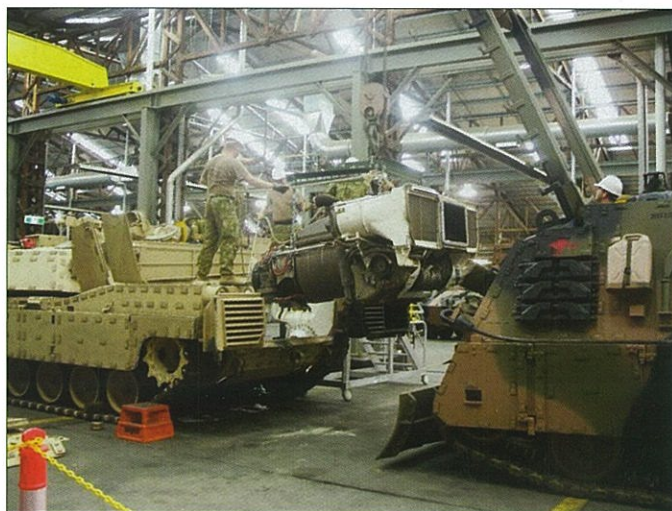
Recce Mechs install an M1A1 power pack using the M88's main boom on the Operator's Course.
