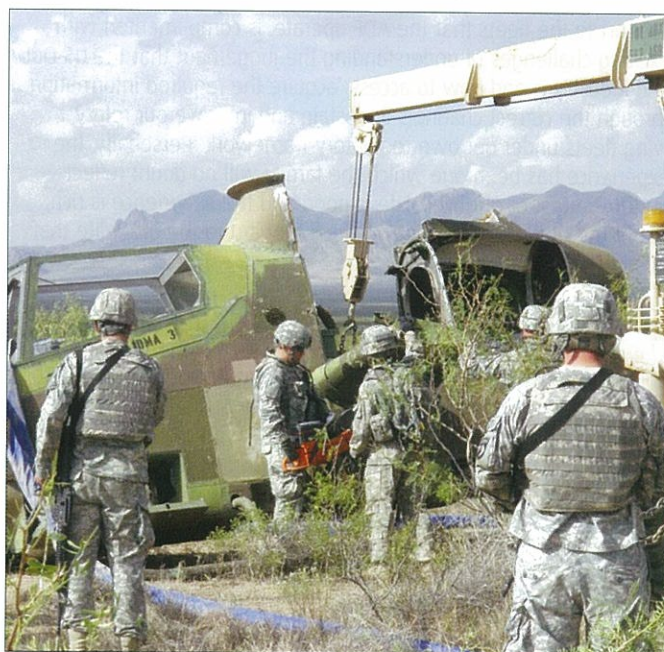
Down Aircraft Recovery Team (DART) prepping to sling a Cobra shell during Operational Preparation Training – FT Bliss Texas
