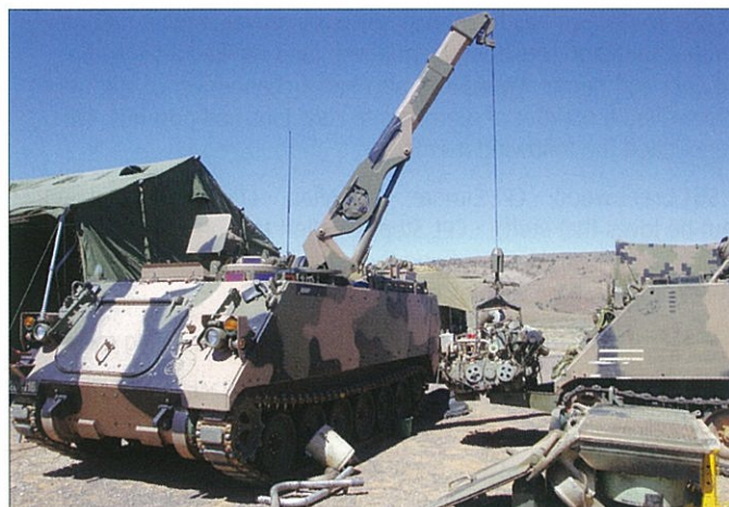
NEW FIXES OLD – An M113AS Fitters doing a pack change for an M113A1 on EX SR 10
