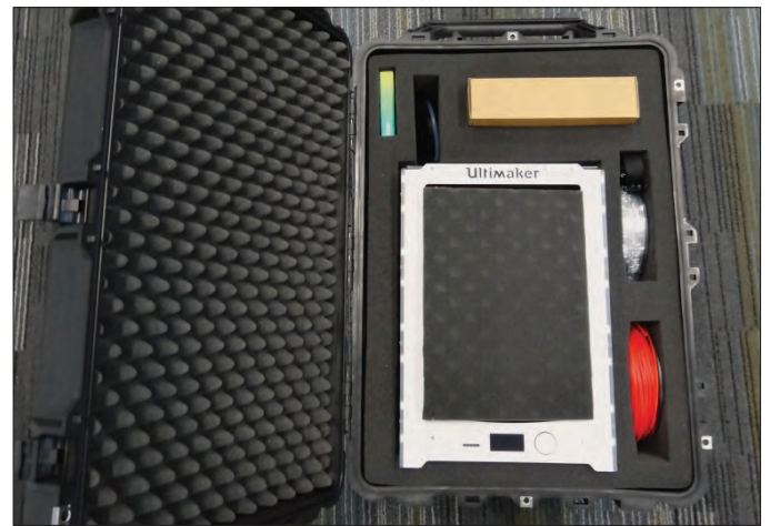
Figure 2. Capability for 3D Printing On-the-move (C3PO).
