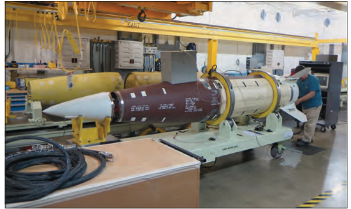
A Letterkenny Munitions Center employee disassembles a US Army tactical missile in preparation for complete inspection of all components.
