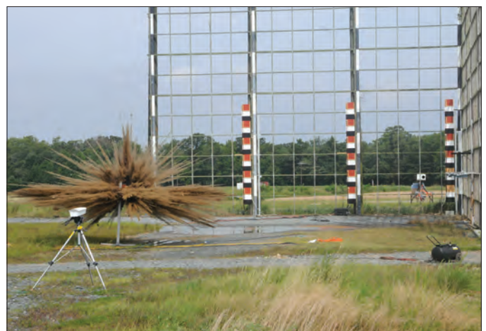
Instrumented testing of a grenade at Aberdeen Test Center.
