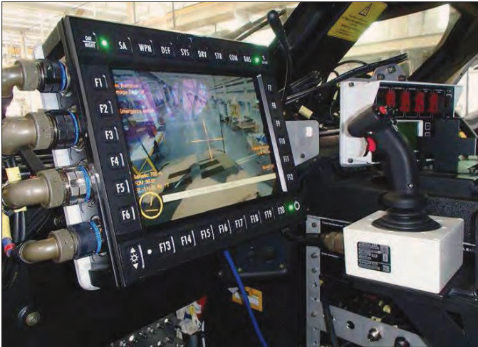
The RWS Display and Hand Controller.
