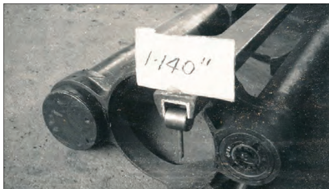
Gauge Maximum Sleigh Rail Depth.
