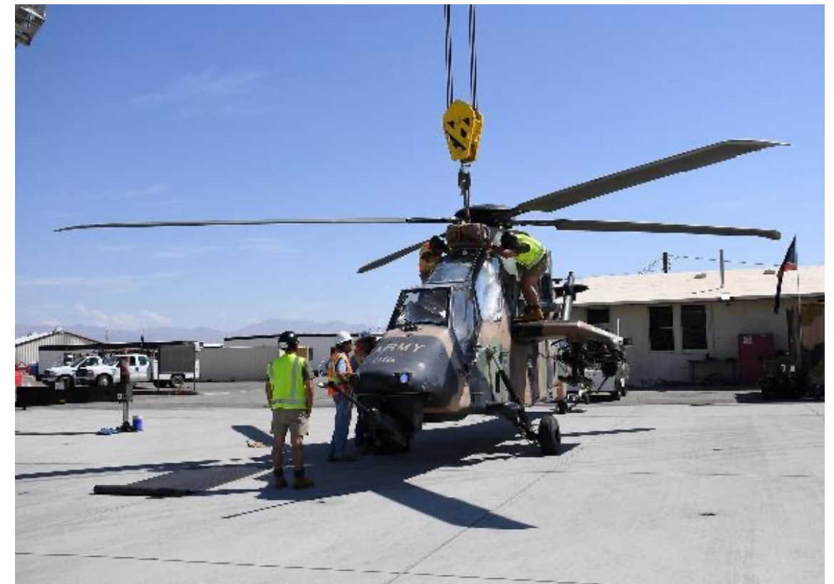
SGT Philip Stokes (Left) supervises the replacement of a Roof Mounted Sight by CPL Dylan Breeze (stubbywing left) and CPL Nicholas Butler (stubbywing right)
