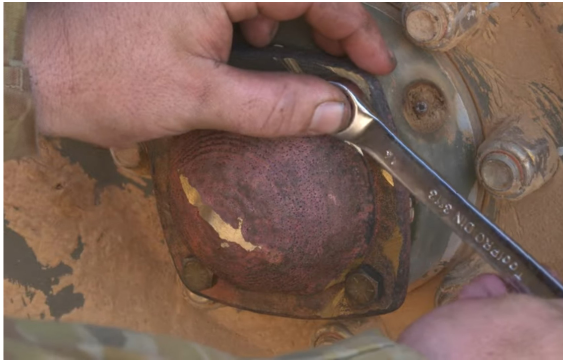
Fitting a wheel bearing cover for M113
