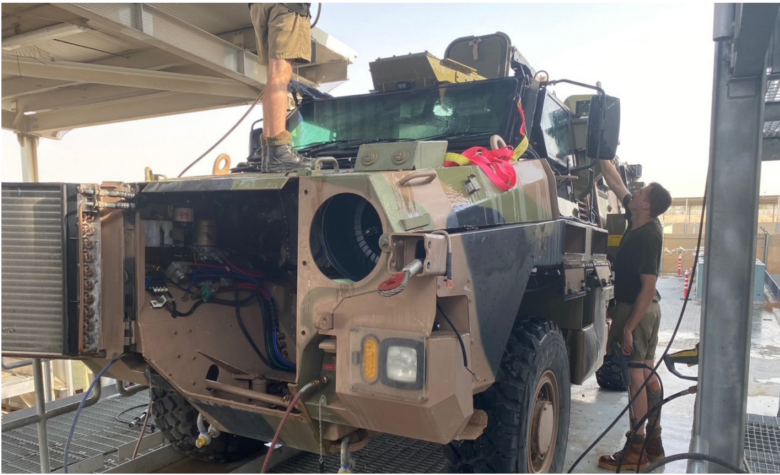
A PMV at the wash point, CFN Whitlock steam cleaning the engine bay
