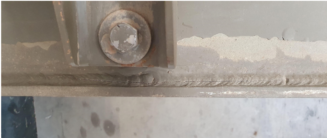
ASLAV spade weld crack
