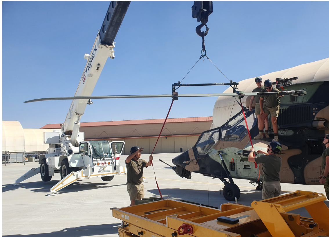
CFN Dylan Wegner (ground left), CFN Kayden Burn (ground middle), LT Harry Foxton (ground right), LT Joel Hobley (stubwing left), and CPL Nicholas Butler (stubwing right) remove blades from an ARH in preparation for return to Australia
