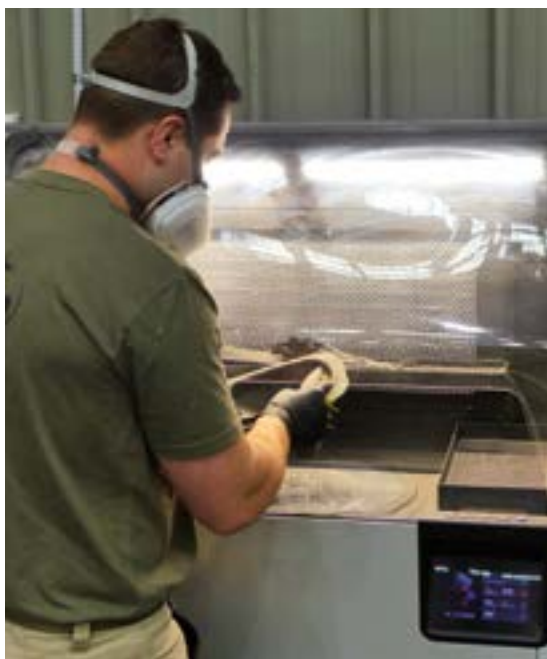
CFN L post-processing an SLS polymer print
